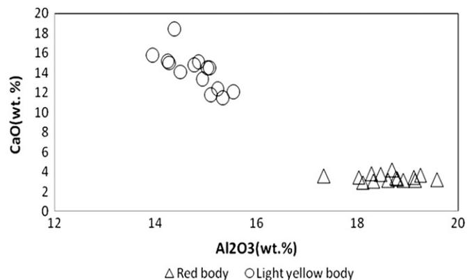
**Fig. 4.** A bivariate plot of CaO vs. Al<sub>2</sub>O<sub>3</sub> content of the bodies.
